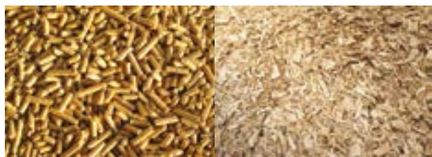
Figure 4: Biomass pellets (left) crushed to flakes (right) using a coal mill/pulveriser.
