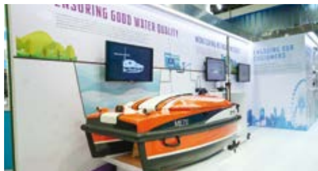
The Autonomous Boat is being test-bedded by PUB to monitor the quality of seawater intake into desalination plants. Photo: Singapore International Water Week.
