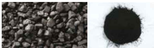
Figure 3: Raw coal (left) crushed to pulverised fuel (right), using a coal mill/pulveriser.
