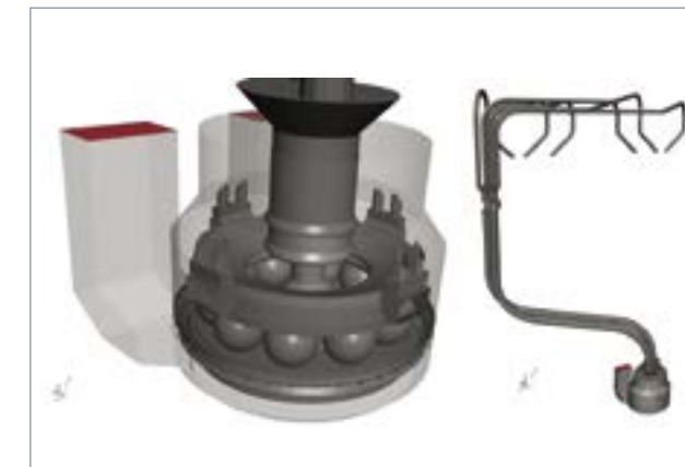
Figure 12: Babcock and Wilcox 10 E vertical spindle mill with the optimised biomass classifier and patented CMP version 4 RT installed. The model includes the pf pipes up to the inlet of the burners.
